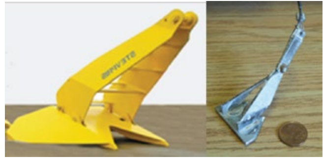
Actual drag embedment anchor, approximately 3 m from top to bottom; Right: scaled drag embedment anchor with “Loonie” for scale
