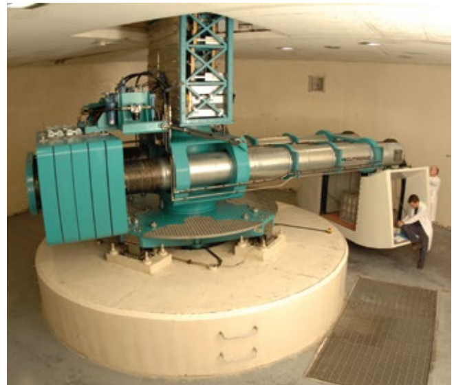
C-CORE's 5.5 m radius centrifuge in Dr. Jack Clark Geotechnical Engineering Building
