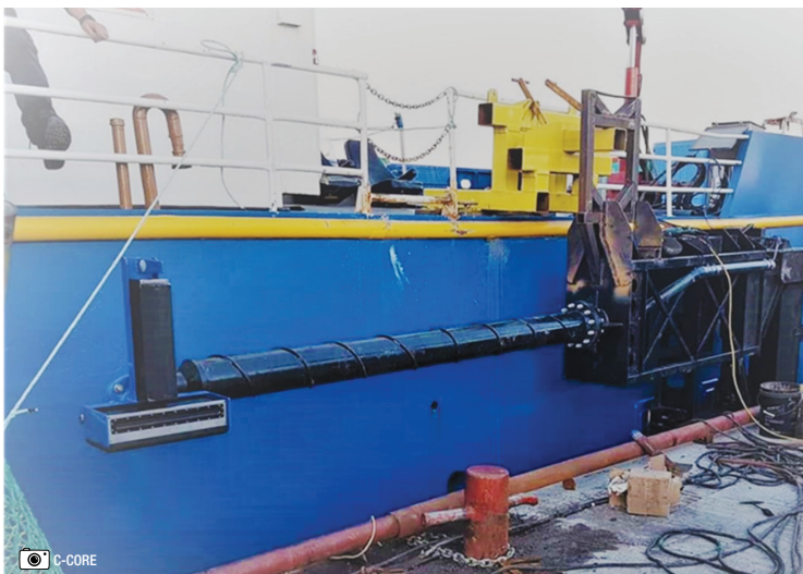
Figure 2: Iceberg profiling equipment – the LiDAR (left) and multibeam attached to hydraulically actuated pole assembly (right).
