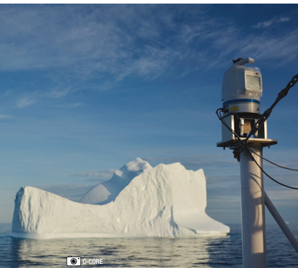
Figure 2: Iceberg profiling equipment – the LiDAR (left) and multibeam attached to hydraulically actuated pole assembly (right).
